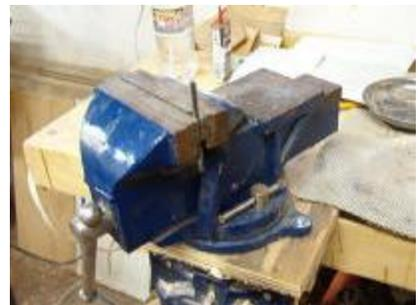
Holding the point of the nail in the vise grips, heat the head and shaft red hot, hold it on the anvil and hit it with the hammer. Continue to turn and hit it, heating it as necessary to form it to the shape of the nail on the right. The head was not cut off. It is faster to heat and hammer it flat.
