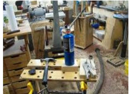
A word about the metal used. I use 2" masonry nails because they are a cheap and easy source of high carbon tool steel. They come hardened and need to be annealed. Just heat them to red hot with the torch and rest them to cool slowly. That is it. Done. I use a fire brick to rest them on to cool but any fire proof surface will work.
