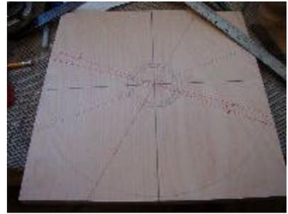
Starting from the center, the trisectors were marked each inch for holes to hold the bowl hold-downs, beginning with the 3 inch mark.
