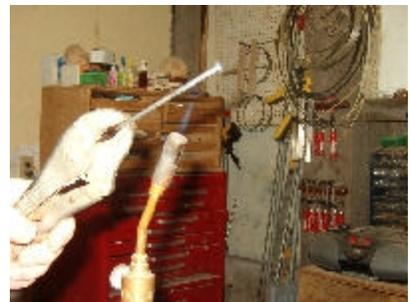
Again using the torch the ends were heated to red hot and hammered flat.
