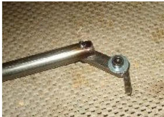
Finally, here it is mounted in a home made arm brace, ready to be used. Any hollowing tool with the cutting tip so far from the angle of rotation will have a lot of torque so an arm brace helps to give control.
