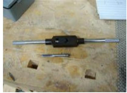
Tapping the hole is like driving a bolt with a wrench when the threads are covered with something sticky. Screw in a turn and back off a half turn. Do it again and again until the hole is tapped all the way through. From time to time add a touch of oil. It goes very quickly at this size. When you are all the way through, back out the tap, blow the hole clear, add a touch of oil and run the tap through a couple of times to clear the threads well. Put in place your bit and set screw.
