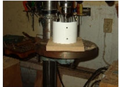
and mark the arm extension at about 10" from the threads to take the self tapping metal screws. Drill the holes
