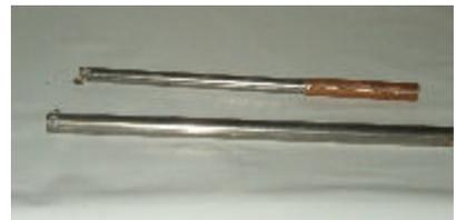
Incidentally, for the limited expansion needed to make the 5/8" shaft fit, an ordinary 5/8" spade bit will work in the galvanized pipe. Wear hearing protection and take your time but it will work. As always, safety considerations are your own.
