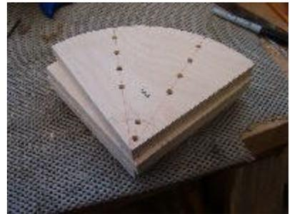
They are mounted to the chuck slides with 8mm machine screws.
