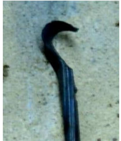
The hook has to be hardened and tempered before use. Heat it red now and plunge it immediately into a bucket of water. Use at least a gallon. This hardens the steel but makes it brittle so it needs to be tempered. Incidentally, I have changed to a regular torch head and a tank that is almost out of fuel. I find a light flame easier to use when tempering such a small piece of steel.
