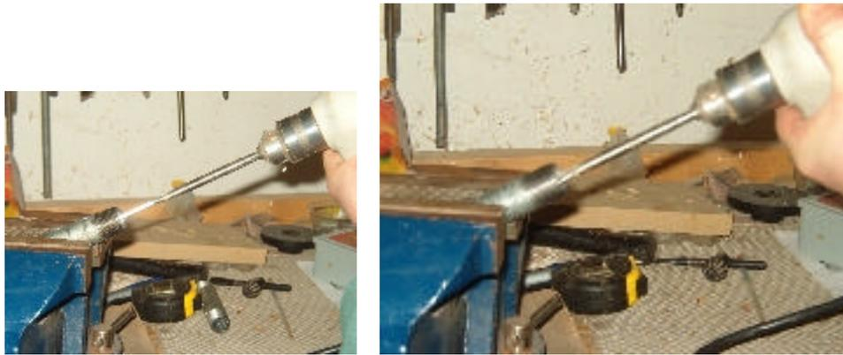
Insert the set screws and assemble tightly the extension to an elbow to the 2" nipple to an elbow to the 4" nipple. You do not want these to rotate under use so tighten hard. Some thin CA trickled into the joints can not hurt.
