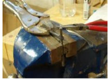
Give it another heat just behind the hook bend it with the pliers to a little less than 90 degrees.
