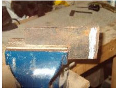
Next I mounted a piece of 5/8" cold rolled steel rod and measured to cut off about 10".
