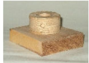
Knock the corners off on the band saw (not necessary but nice) and mount to the lathe.
