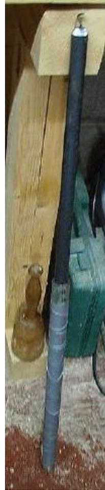
And these are a couple of the hooks that I use. If you plan on using a commercial hook or ring, just drill the appropriate holes in the shaft. It is easy to make the shaft double ended. Drill and tap the other end and flip it in the handle.
