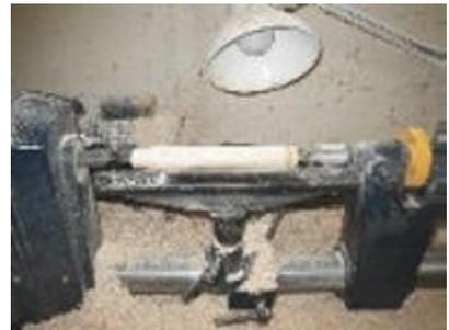
Drill a 3/8" hole in the business end of the handle. I use a jig in the drill press for this but if you hold the handle in a bench vise and take your time, a hand drill will do. About an inch should be sufficiently deep for this tool. While the temptation is to bury that tool shaft as far as possible, it turns out that many of the tools we use have from one to four inches of shaft in the handle and an inch and a half is far more common than four inches.
