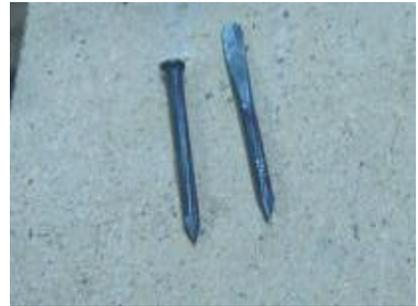
Now to the grinder. I want a hook with an inside bevel for the particular cuts I am about to make. An outside bevel is usual and the one I use the most. As you look at the nail with edge up ward, for an outside bevel grind it on the left, for an inside grind it on the right. Here it is ground on the right. I first grind the edges straight, then the sides flat, then the bevel to about 45 degrees.
