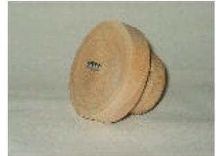
I like to cut off the tip with a Dremel or similar. The chuck is typically used with a pre-drilled hole and the point is not necessary.
