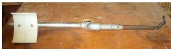
Not able to leave well enough alone, I made a few changes. First of all I made a shorter arm and then changed from hex cap bolts to a pan head for the cutter and flat head for the arms. I also countersunk for for the flat head screws. Here is, starting from the upper left, the cutting tip, washer, pan head screw, flat head screws, short arm, long arm, and shaft.
