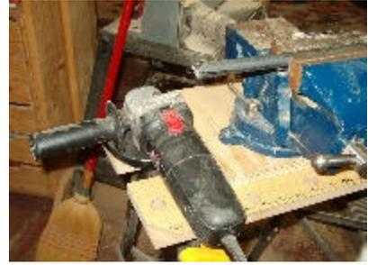
Using a 4 1/2" angle grinder I cut a flat about 1/2" wide and a bit above the diameter of the rod and made it about. If you do not have an angle grinder you could grind it at your sharpening grinder.
