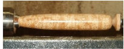
The handle is removed from the lathe and mandrel
