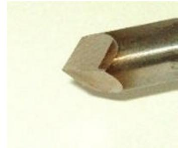
Repeat the grinding with each of the remaining sides to give a tool with a center point and three cutting edges.
