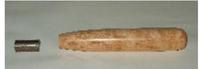
and the insert pressed and glued into place.
