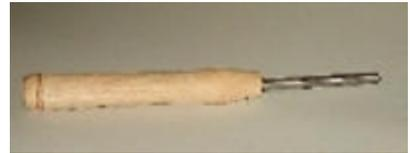
Mark three evenly spaced dots around the perimeter of the shaft end and a dot in the center. Let us go to the grinder. Set your grinding table to about 150 degrees and with the two of the points parallel to the ground, i.e. the surface of the wheel, grind to center. You now have one mark opposite a flat. The edges of the flat are your other two marks.
