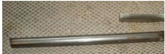
The bar is cut to 2" long and the ends slightly rounded.
