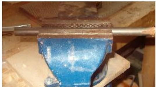
Here are a couple of shots of the receiving platform ground to about the half way part of the rod and about 7/8" long.
