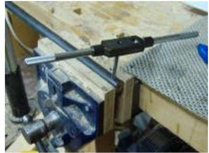
Do the same drill and tap procedure to the galvanized steel handle about 1/2" and 1" back from the end. I am cheating a bit here as I am using the same handle that I use on my 3/8" Oland tool. The duct tape makes it a bit more comfortable for me especially on cold days.
