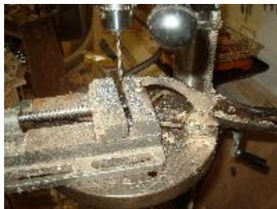
Rotate 90 degrees and drill a 13/64" inch hole to tap for a 6 x 1 mm set screw or adjust for the set screw of your choice
