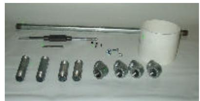
Set the pvc coupling on end and run it through the band saw to give 2 arm rests.
