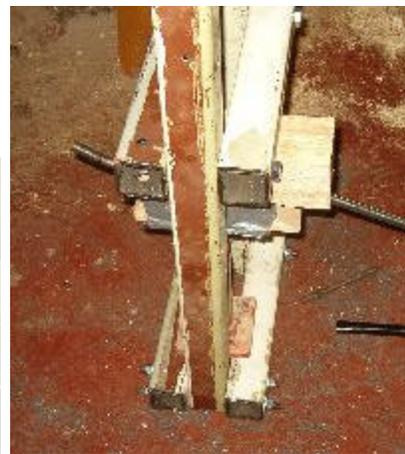
In goes the steel and the jack is slowly raised for the first bend. Some careful positioning and the second bend is accomplished. Then I checked it with my sketch and realized a bit of tweaking was needed. I decided to bend it a bit at the point where the arrow directs.
