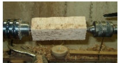
and turn the handle to a comfortable fit. Normally I like unfinished tool handles but this being a present, I used some turner's polish to finish it.
