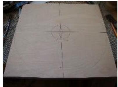
A little more geometry and each quadrant was divided into thirds, complete with an easily corrected error.
