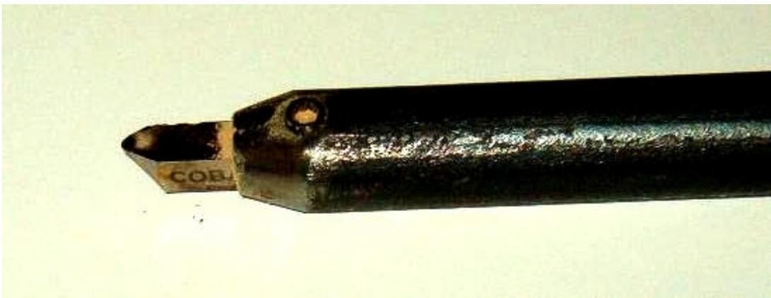
As you can see I have drilled and tapped for a set screw about 1/2" behind the tip. I find this sufficient to hold the tip in place although you might want to put another set screw about 1/2" behind the first. Out of habit I use 6mm x 1 set screws but 1/4" x 20 would work as well. I have also ground the end of the shaft back to give a bit more clearance for the cuts. The tip is ground to about 45 degrees and is usually more rounded than I have it
