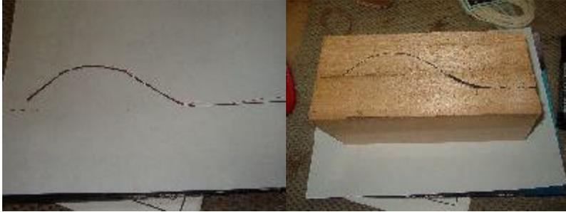
The sketch was transferred to a block of maple and cut out on the bandsaw
