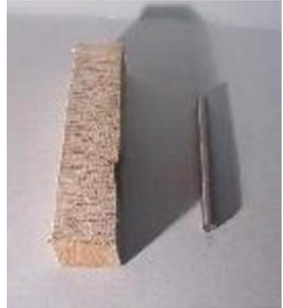
Mount the wood for the handle between centers and turn to your favorite handle shape. If you are not sure what that is, try the feel of a couple of your lathe tools and shamelessly copy the one you like. I am using my monotube lathe from Canadian Tire and turning about 2500 rpm.
