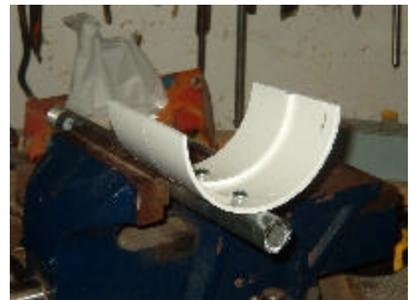
The general problem with this is that the pipe that is easily available to me does not quite fit my turning tool shafts. It is a bit too small for a 5/8" and a bit too large for 1/2". I drilled it out for the 5/8" and shimmed the 1/2" with copper pipe, grinding it away until I had a fit.
