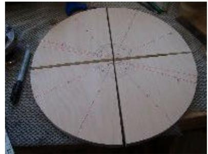
After drilling 1/4" holes for the hold-downs and 8mm holes for the jaws, there are four jaws ready to go.
