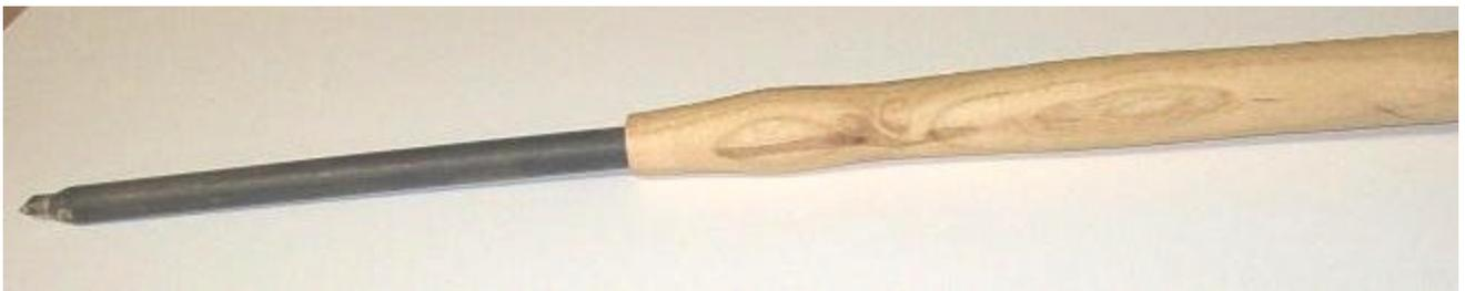
This is a shot of my 1/4" Oland Tool. Note that this is a working tool and nothing was done to make it fancy for sale. I turned a handle about 14" long and drilled a 5/8 hole about 2 1/2" deep into it. The shaft is cold rolled steel with about 10" extended from the handle. The tip is a 1/4" x 2 1/2" HSS cutting tool, standard in the metal lathe industry.
