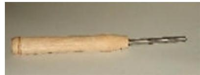
A three point tool is used like a skew but without some of the dig in dangers. Bill Jones, the third generation English turner, is a strong advocate of the tool especially in small spindle turnings.
