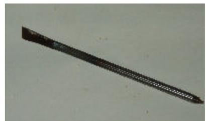
The cutting edges are then hardened by heating each tool to red hot and immediately quenching in water. After each edge is polished so as to be able to see color changes, they are tempered by heating with the torch to straw color and immediately quenched in water to stop the color change.
