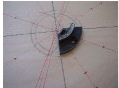
Then to the bandsaw and the circle and jaws are cut ready for drilling.
