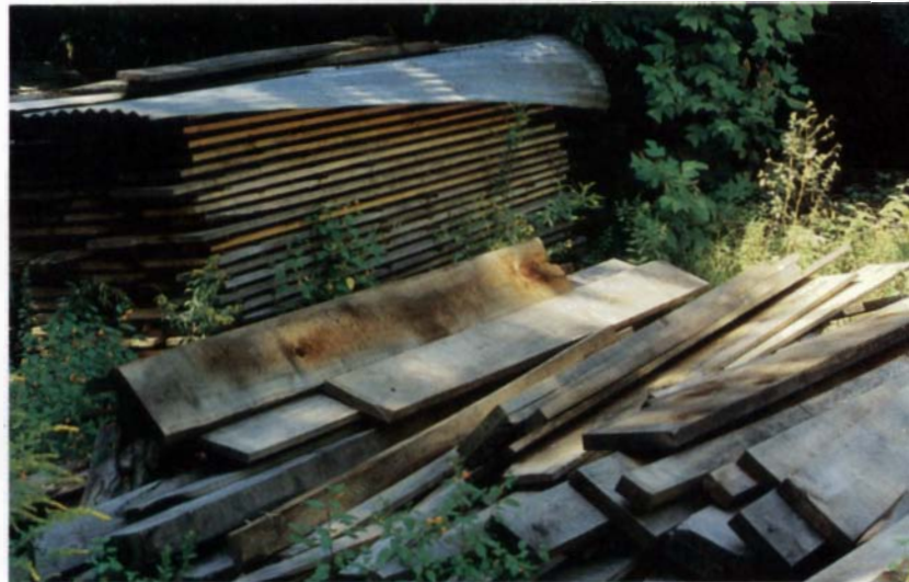
Sawyers can get so busy that they often don't have time to properly stack the lumber they've sawn. The back stack is good, but steer clear of lumber piled like that in the foreground. Lumber from such piles often contains a high percentage of cracked, cupped, bowed and twisted boards.
