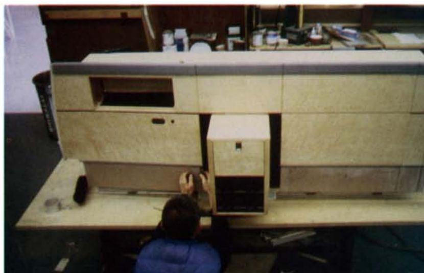
The forward bulkhead—the largest cabinet built—required more than 2,000 man-hours. Its drop-leaf desk, hidden stereo and rotating refreshment bar (with icebox) were operated by solenoid switches.
