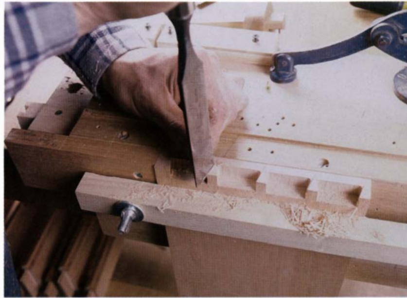
The router does the hard part by precisely locating the width and depth of the sockets, which can then be squared by jiggling a chisel against the routed surfaces and slicing down to the corner.
