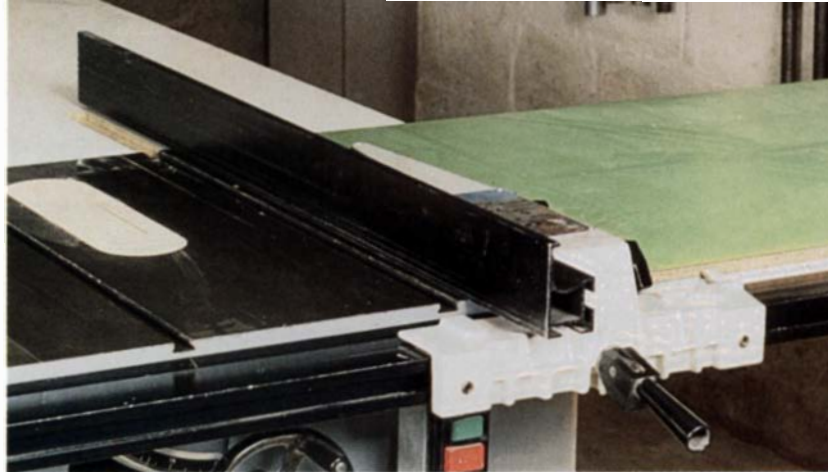
The fence bar on Delta's Unifence slides forward and back, and can be dropped all the way down to the saw's table so thin laminates won't sneak underneath during cutting.
