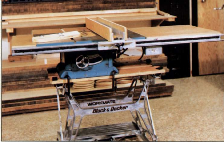
Made of stock aluminum and steel channels, the author's homemade rip fence bolts together and can be customized to fit any tablesaw or machine tool.
