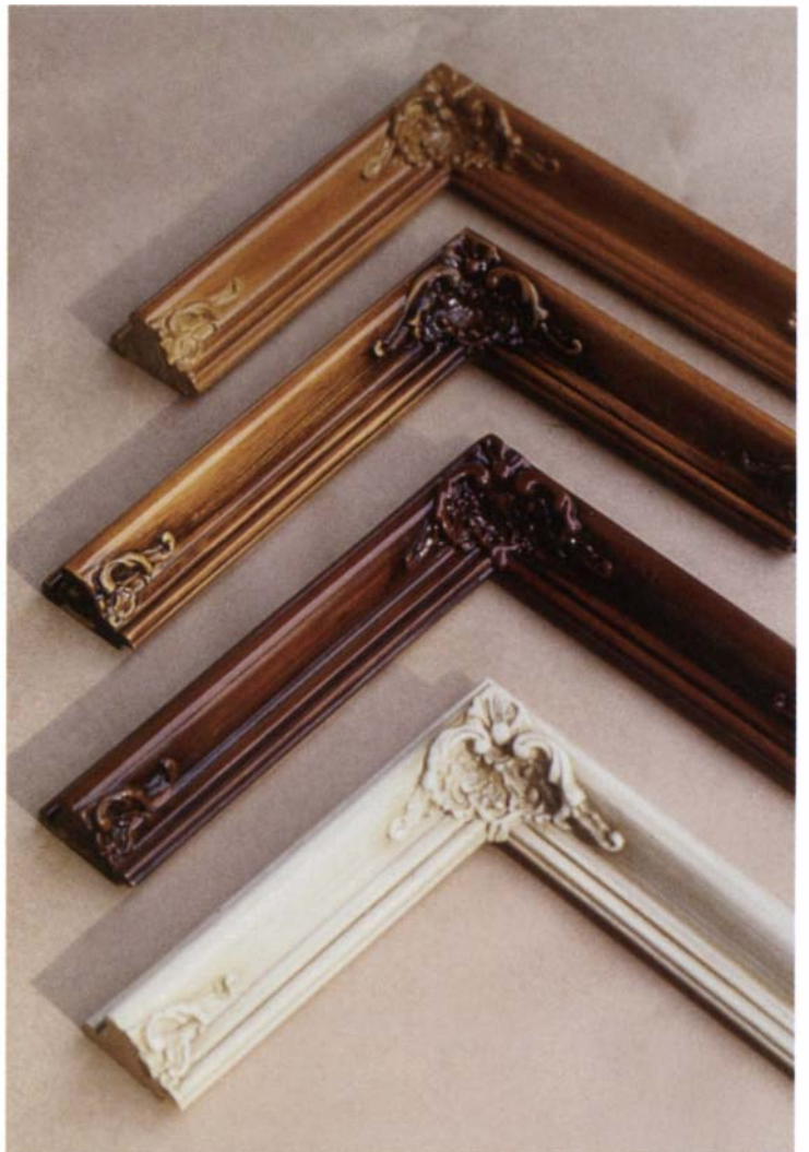
These four frames illustrate several ways of using shading, glazing and toning in combination. From top to bottom, the frames are: stained light walnut; glazed with brown and clear-coated; toned with tan, glazed with brown, shaded with maple and red and clear-coated; toned with white and glazed with raw umber.
