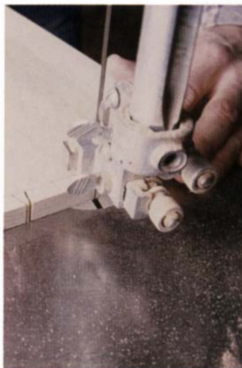
The tails are bandsawn freehand (left). A fine, smooth cut comes from using a blade whose set has been removed by running it against an oilstone. The waste is then chopped out (right).
