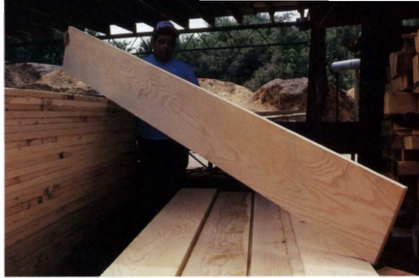
Dick Pawloski, a sawmill operator in Bethel, Conn., hefts a flat-sawn FAS 4/4 oak plank fresh from the mill. The board has been edged, trimmed to length and graded, and is ready for drying.
