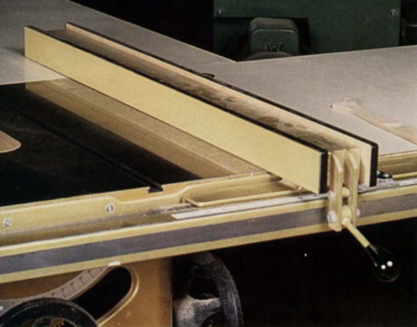
Except for its laminate-faced auxiliary fences, the Biesemeyer fence is built entirely of steel and is an available option on the Powermatic model 66, shown here.
