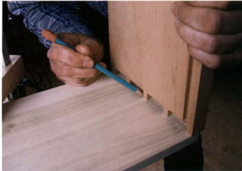
The tails are scribed from the routed pins in the usual way.
