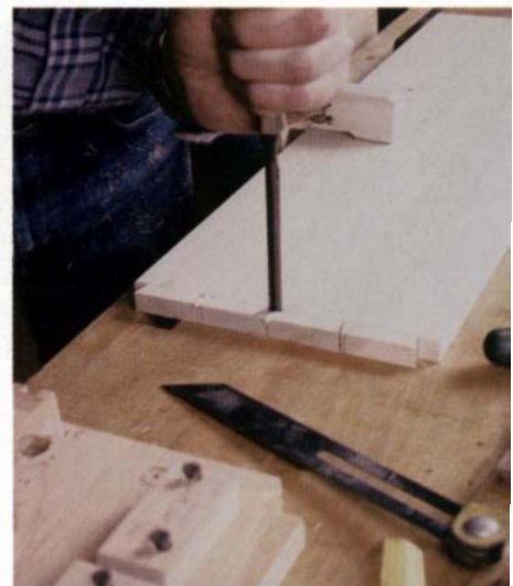
The tails are bandsawn freehand (left). A fine, smooth cut comes from using a blade whose set has been removed by running it against an oilstone. The waste is then chopped out (right).
