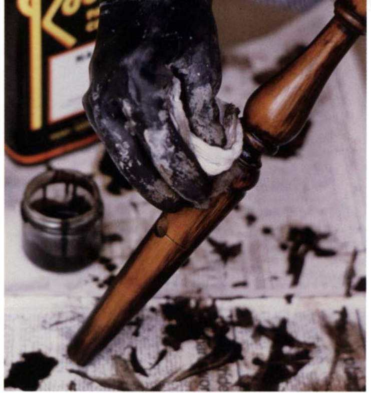
It's not critical to apply a glaze evenly, since most of it is wiped off the prominent surfaces before it dries. The pigment left in the recesses can create contrasts to highlight carved and turned details or give a piece an aged look.
