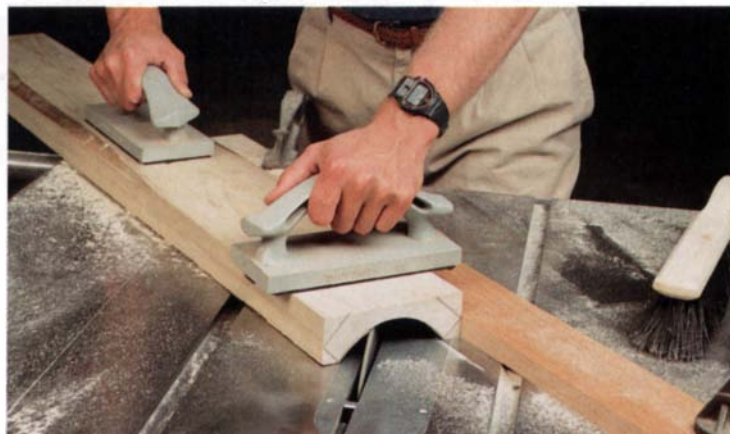
Symmetrical coves are cut with the blade vertical. Klausz shaves the last 1/16 in. from a piece of symmetrically coved cornice molding. The fence is set up to the infeed side of the blade, so the cutting action holds the stock against the fence.
