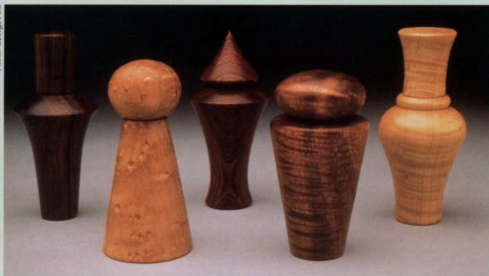
Fast finish —Sage's production methods include a one-step finish borrowed from a jeweler: He brings the 4-in. bottles to a sheen with carnauba wax on a buffing wheel.
