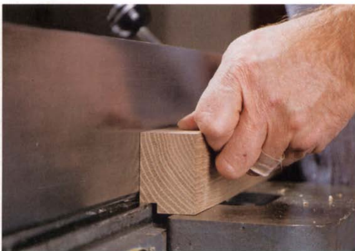
Clean rabbets —With the fence set near the jointer's edge, the author slides a piece along the rabbeting arm, taking \frac{1}{16} in. at a pass. For clean rabbets, all the knives should project equally toward the rabbeting-ledge end of the cutterhead. A few woodworkers sharpen the ends of the knives to further improve the cut.
