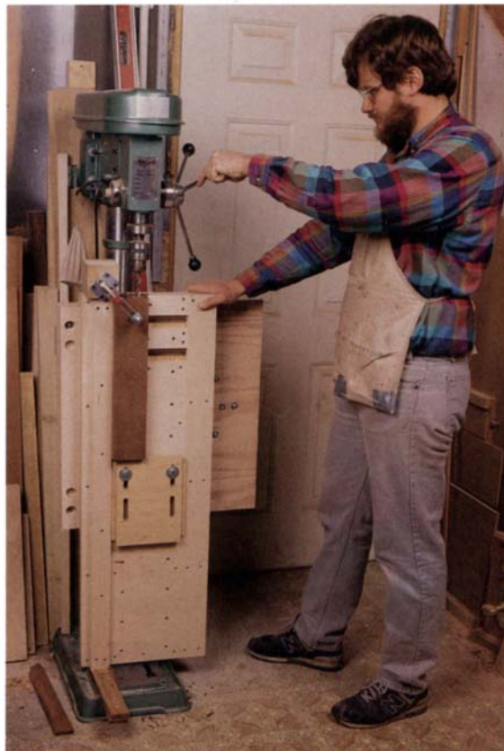
Boring the ends of long workpieces used to present problems for the author, Jeff Greef, until he devised this end-boring jig for his drill press. A pair of platens mounted to the press's table allows adjustments in and out and left and right.
