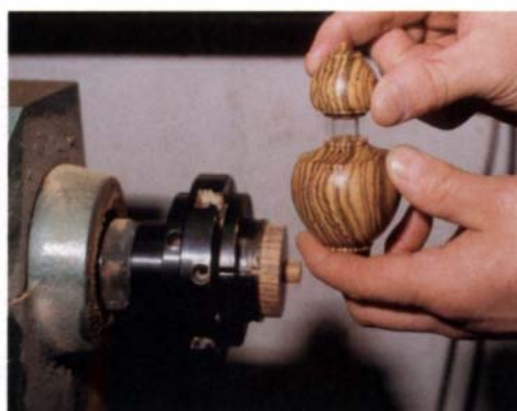
Aligning the grain—With the cap already glued hard, Christensen presses the vial into the base, being sure to align the grain.
