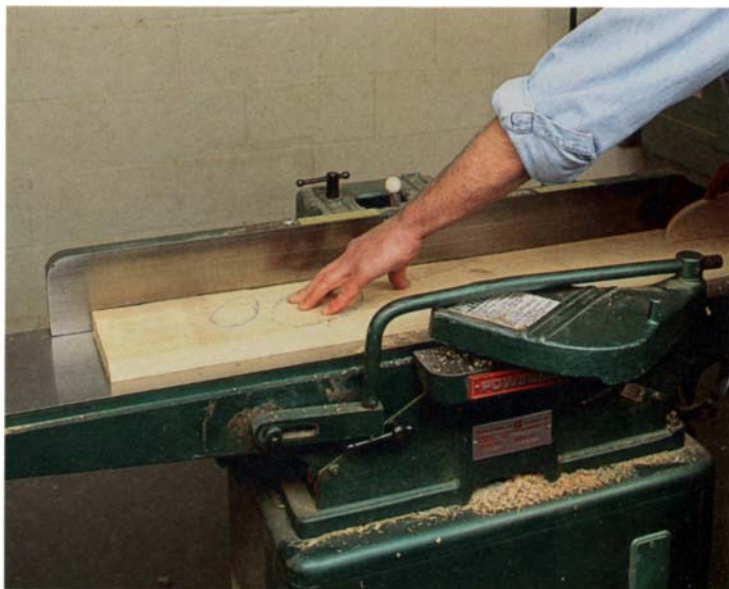
The first step in stock preparation is to create one flat face, which becomes the reference face. So long as your jointer's capacity is greater than the width of the board you need to flatten, it's a quick operation. Whenever you joint, maintain pressure on the outfeed table just past the cutterhead. Always use a push stick.
