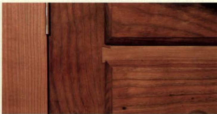
The thumbnail molding around the drawer fronts adds just a bit of restrained ornament to this well-designed but utilitarian bench. The molding is easily cut with router and tablesaw.
