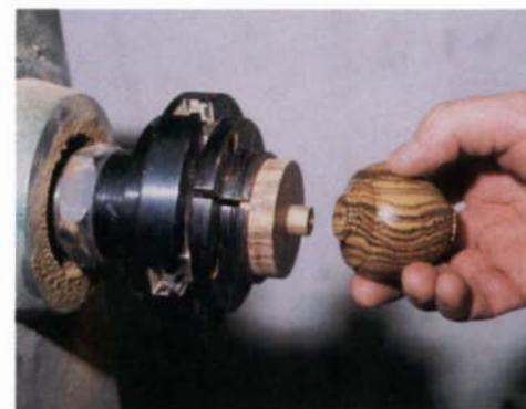
Quick flip —The parted off and lacquered base is remounted on the waste piece to clean up the bottom.
