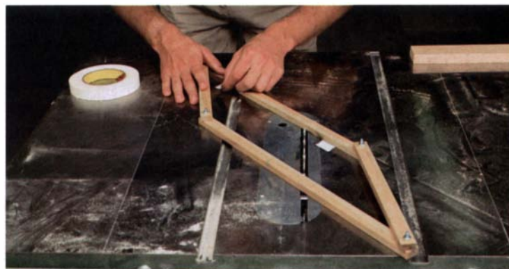
Klausz finds the angle of approach for a symmetrical cove with a parallelogram set to the cove's width. With the blade raised to match the cove's highest point and the parallelogram just touching the blade at front and back, he marks the front fence location.
