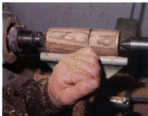
Parting the blank —Christensen separates a blank of bocote into base and lid. A Nova chuck will lock onto the end spigots.
