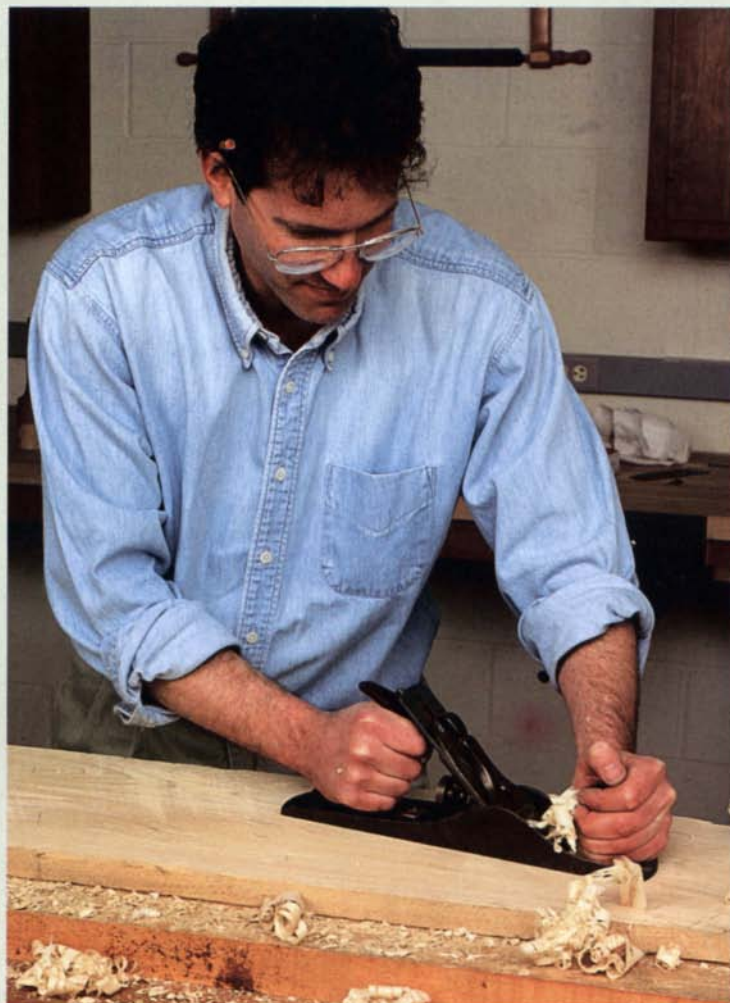
Taking a bench plane and planing with the grain, Korn takes out the scrub plane's marks and smooths the face of the board flat, readying it for the thickness planer and further milling.
