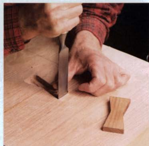
4) Pare to the line, and clean up the corners with chisels.
