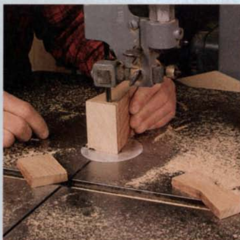
Cherry butterflies —Vogt bandsaws a stack of keys from a block of cherry.
