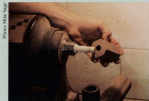
Mounting the blank —With his chuck seated in the lathe's taper recess, Sage mounts the predrilled blank.
