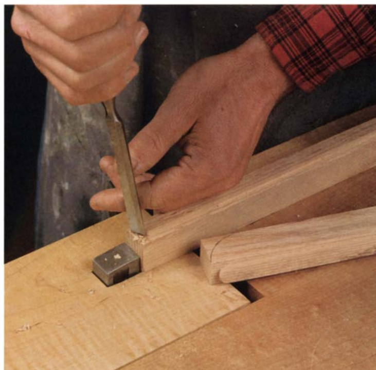
Rounding off the dovetail tenons —After shaping the upper rails' dovetails on his router table, the author uses a \frac{1}{2} -in. straight chisel to trim the ends. Rounding the ends ensures that the dovetail tenons fit the stopped grooves in the underside of the top. Next Vogt will bandsaw the curve marked on the rail.
