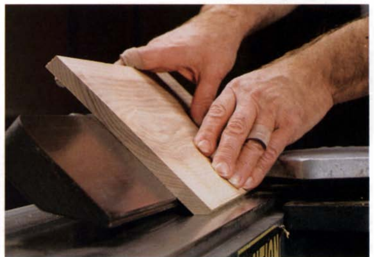
Smooth chamfers and bevels —A jointer is more versatile than you might think. For decorative table legs, for instance, you can chamfer the corners on the jointer. Or you can precisely bevel staves for a planter. Just angle the fence, adjust for a shallow cut and then feed the work edge over the jointer in several passes.
