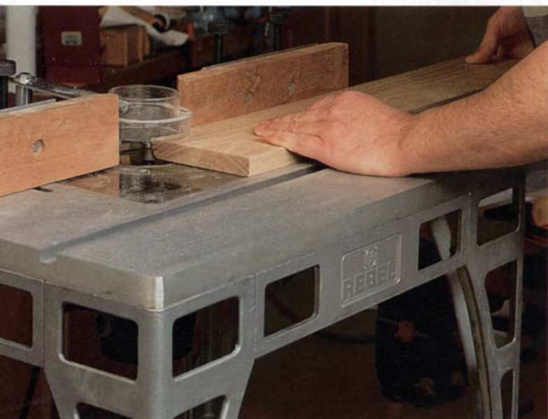
Cast aluminum tabletop, legs and stretchers give the Woodstock International W2000 Rebel a solid chassis. Because of its 17-in. height, it's best used on a dedicated stand.
