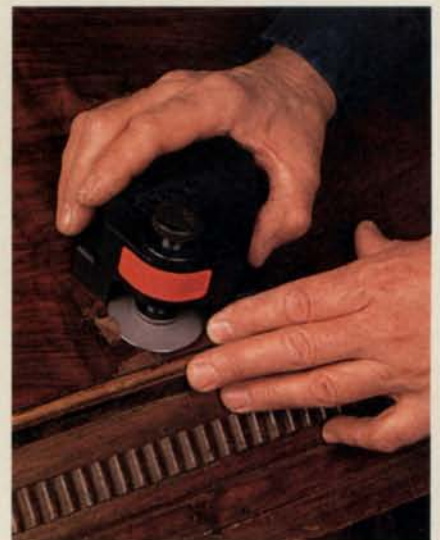
Trimming burn-in repair material flush is done without fear of damaging the surrounding finish, thanks to the Ieroplane. The Ieroplane is included in Mohawk's new Concept 2000 repair system, which makes burn-in repairs easier for the beginner.
