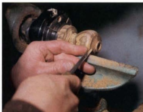
Shaping the base —The author uses English-style spindle gouges on edge with the flute to the side to cut fine details.
