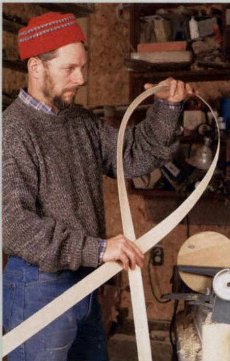
Strong and flexible, thin strips of tulip can be bent in relatively tight circles without cracking, as demonstrated by the author.
