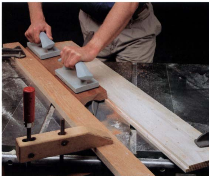
A stepped fence raises one edge of the workpiece as Klausz cuts a partial cove in a piece of cherry. For all asymmetrical coves, partial or full, two fences are required, and the stock is fed into the acute side of the blade's tilt.
